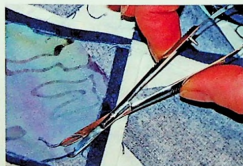
Famoré™ 4.5" EZ Snips™ with "hook" feature for picking out threads and snipping as well; although not a serrated blade on this model.
